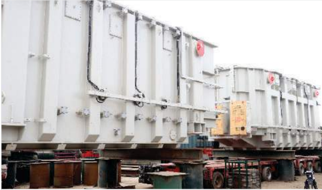
2x100/125MVA power transformers and accessories at Alagbon 330/132/33kV Transmission Substation.
