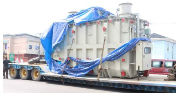
60MVA power transformer and its accessories at the Rumuosi 132/33kV Transmission Substation in Port Harcourt.
